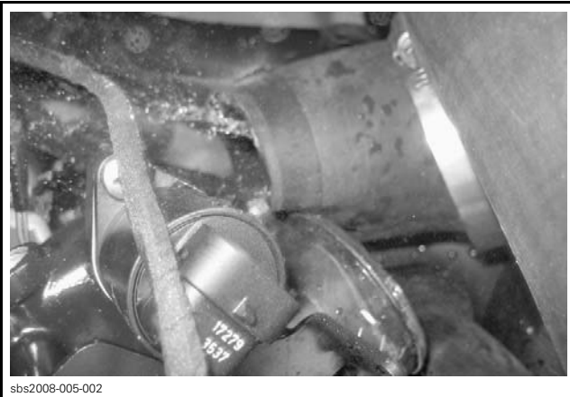
sbs2008-005-002 WATER EXPELLED FROM INTERCOOLER
